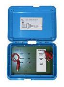
**Calibration box** for conductivity measurement (conductive) with simulation resistances for the measurement ranges 0 - 2, 0 - 20, 0 - 200 μS/cm
